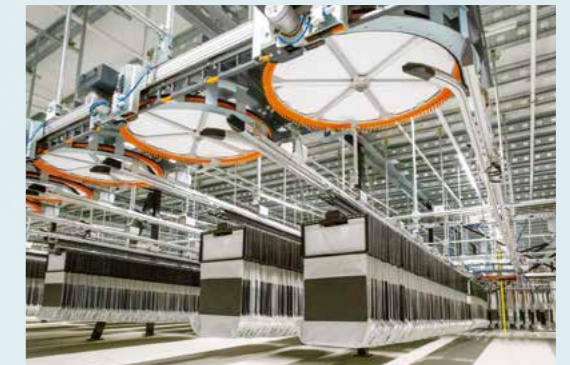
Vanderlande's hanging high-speed sorting system
