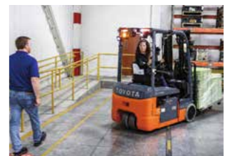
Three-wheel electric lift truck to which operator assist and other functions have been added
