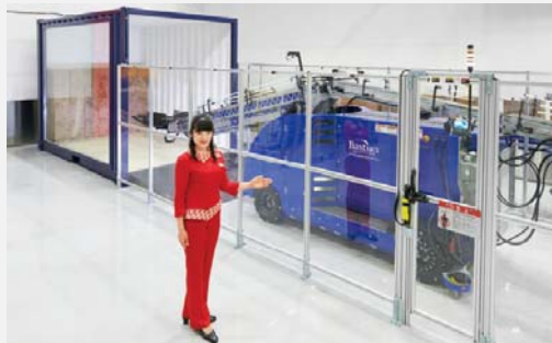
Automated loading robots to a commercial truck, "ULTRA"
