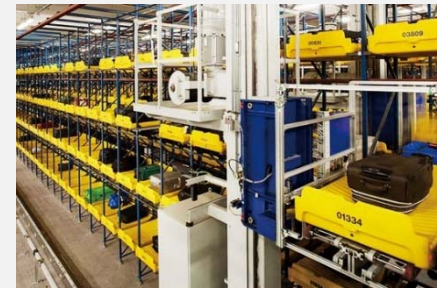
Automated warehouse for baggage
